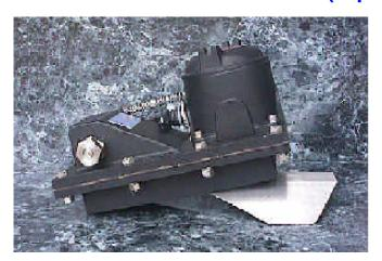
The 97ZB0004 Mud Flow Sensor is a paddle type sensor that monitors mud flow through the return line. The sensor is mounted on the return line with the paddle extending into the mud flow. Deflected by the force of the mud flow, the paddle drives a potentiometer which produces a DC analog signal that is proportional in amplitude to the position of the paddle. This voltage can be used to monitor, display and record mud flow information.
