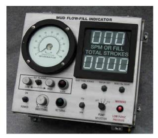
The Mud Flow-Fill Indicator displays mud flow rate and pump stroke rate or fill count and total strokes during drilling or tripping operations. The indicator displays return mud flow status (0 to 100%) on a 5 1/2" analog flow meter.
